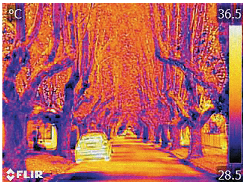
Figure 2: Thermal image of an urban street with large trees. The surface temperature is indicated on the right of the image in the scale bar. (Courtesy Banyule City Council, image © ENSPEC).
